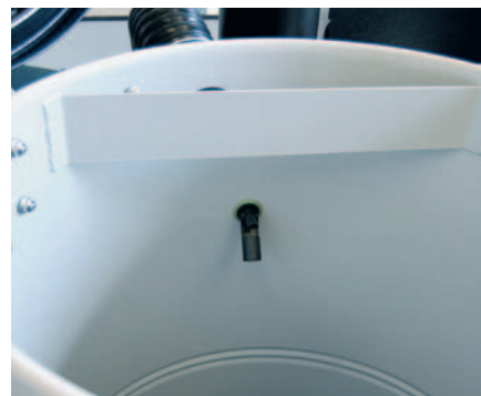
AUTOMATIC LEVEL CONTROL
